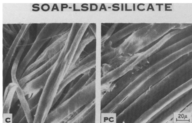
FIG. 1. Photomicrographs of cotton (C) and polyester-cotton blend (PC) fabrics washed 25 times in hard water containing 0.2% of soap-LSDA type detergent.
